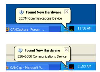
Subsequently a bubble should appear at the bottom of your computer screen message will appear stating that the drivers are installed and the new hardware is ready to use.
